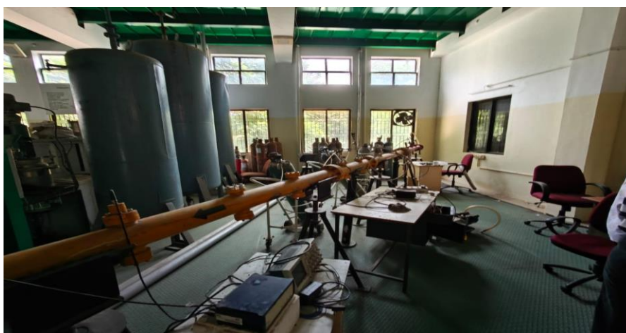
Figure 1: Schematic diagram of the shock tube experimental setup used for high-enthalpy oxidation testing
