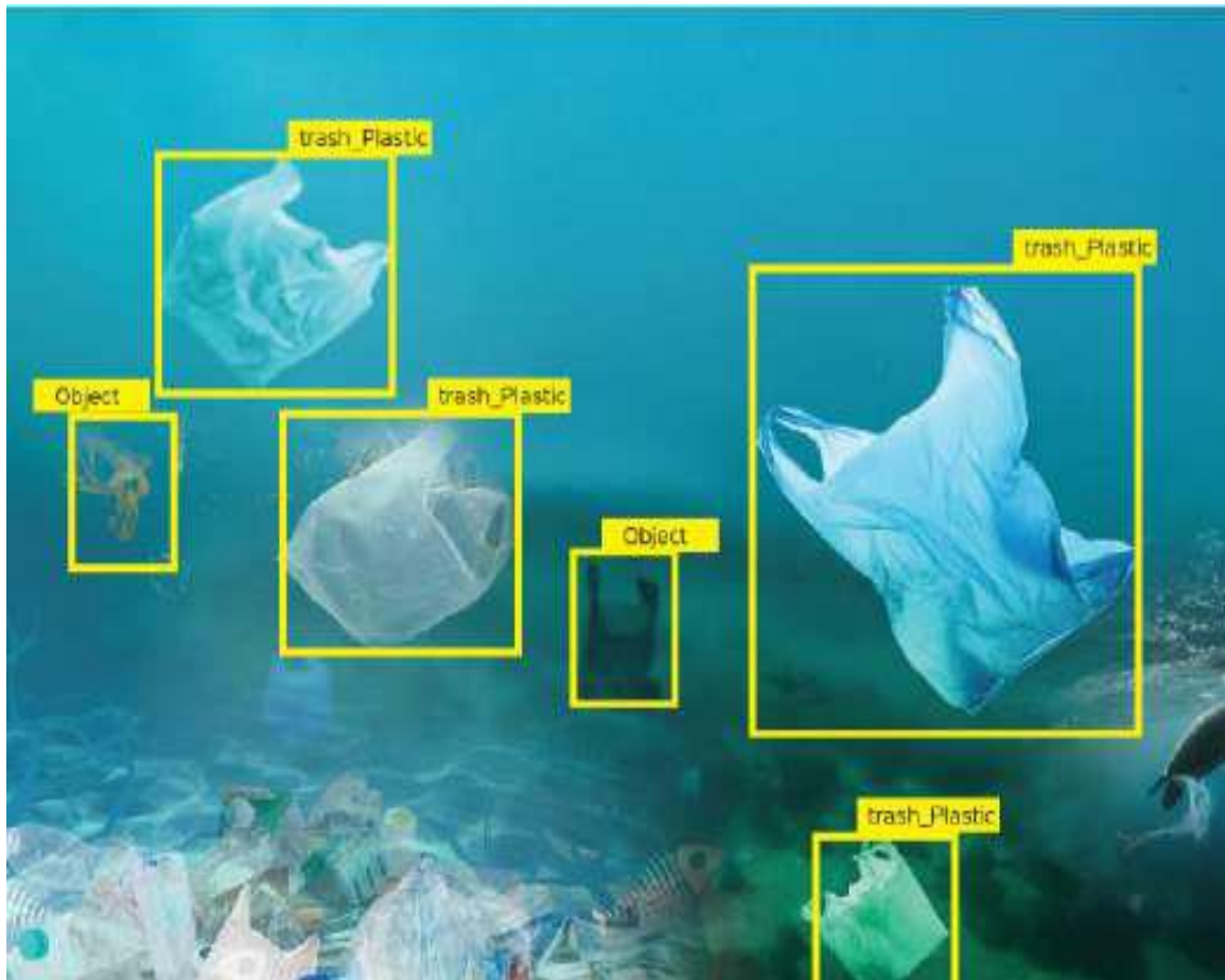
Figure 1: Detection of marine debris and plastic waste using YOLO-based underwater object detection
