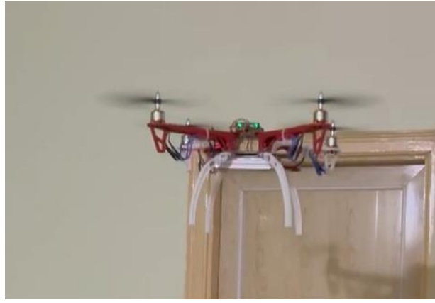
Figure 3: Hover-Level Integration Test for UAV
