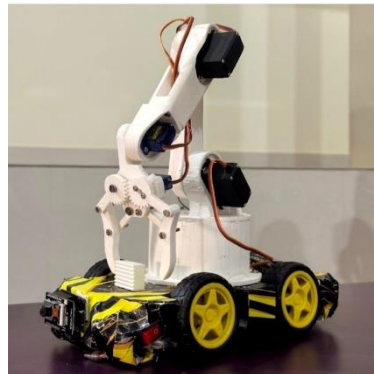
Figure 1: Wireless Bioni Arm on Robotic Vehicle Project Module
