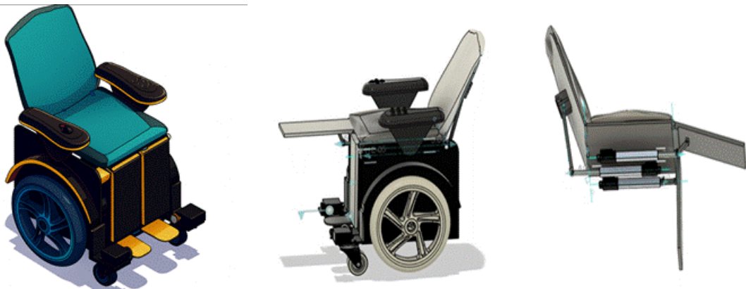
Figure 1: Finalized 3D CAD Design of the Biomechatronic Smart Wheelchair Created in Autodesk Fusion 360
