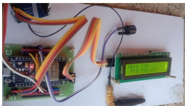
Output Display When Heart Rate Sensor Is Not Working
