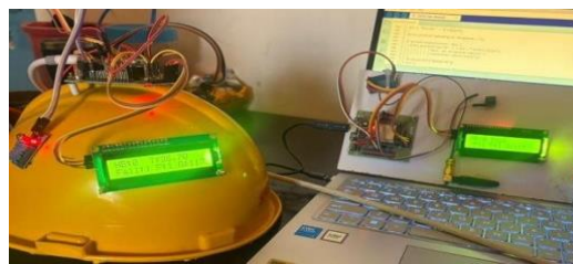
Prototype Output Showing Normal Heart Rate and Gas Levels
