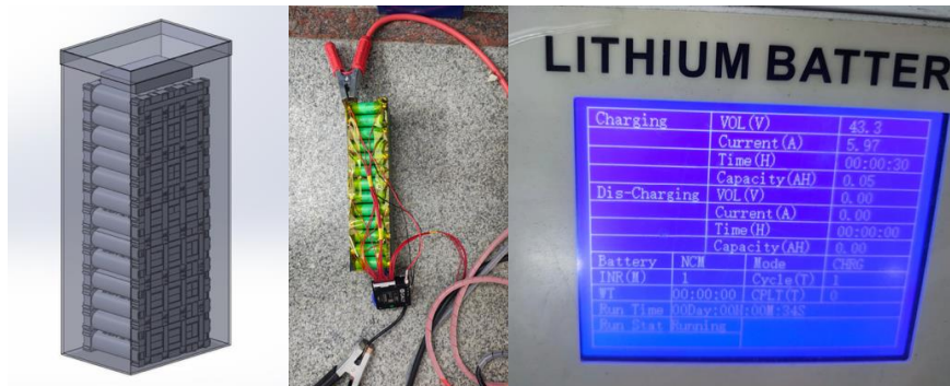
Figure 2: (a) CAD model of battery pack, (b) fabricated 21700 cell assembly with BMS, and (c) real-time charging data from battery testing unit.
