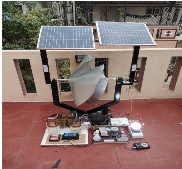
Figure 1: Proposed model of the integrated solar-wind renewable energy system
