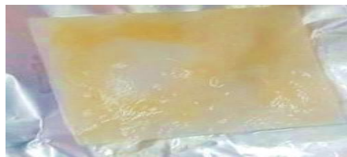
Figure 6: Sample paper which is impregnated with potassium permanganate ( \text{KMnO}_4 ) and dried under dark conditions. 1mL of phosphoric acid along with 1ML of 1mg/ml sample was added and
