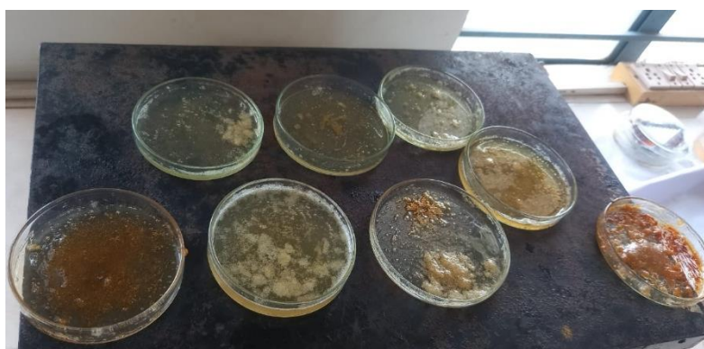
Figure 2. Collected gel was dried using hot plate, to get pectin pellet.
