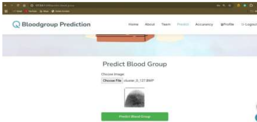
Fig 6: This figure represents that users are allowed to select the fingerprint image from the dataset and upload it to the website.
