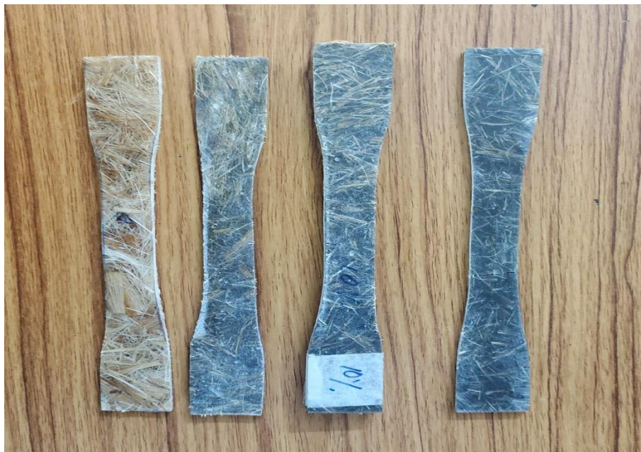
Figure 1: Bio composite specimens (PLA, Flyash & Pineapple leaf fibers)
