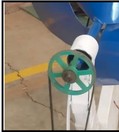
Figure 7: Grooved Large Pulley (91mm dia)
