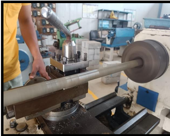
Figure 4: Selection of aluminium shaft (1 inch diameter)
