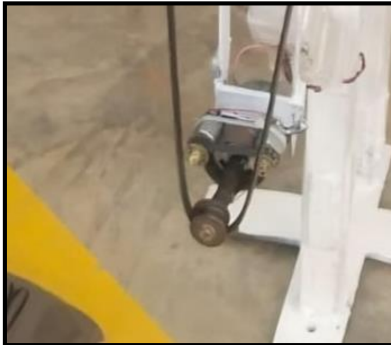
Figure 22: Integration of 12V and 5v DC motors
