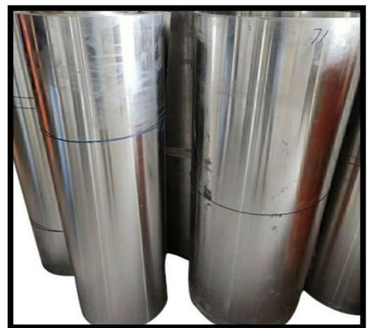
Figure 3: Selection of aluminium sheet (0.9mm thick).
