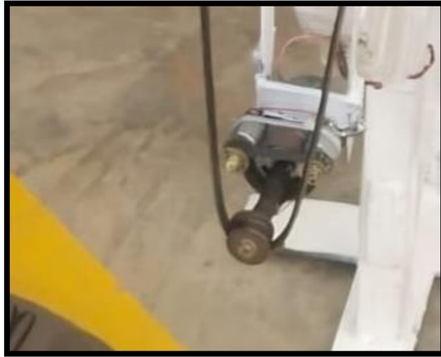
Figure 8: Small Pulley (51mm dia)
