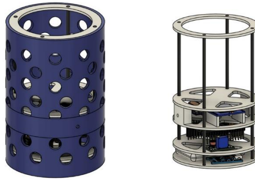
Figure 2.1: Structural and Internal Architecture of CAN Satellite
