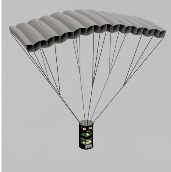
Figure 1: Structural CAD Model of CAN Satellite with Parachute-Assisted Descent Mechanism
