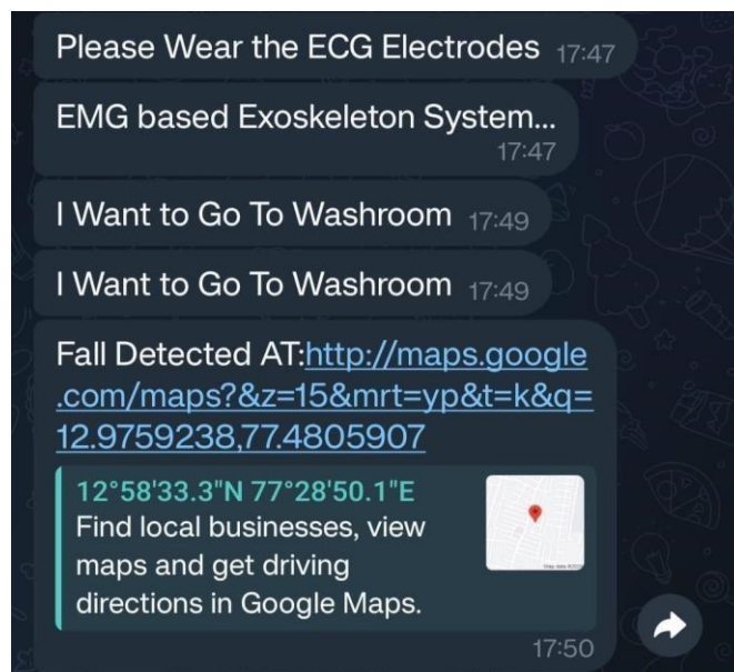
Fig 6: Message of Fall detection and Gesture detection to Care Take in Telegram
