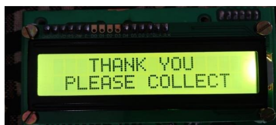
Fig. 2 (e): LCD display to Collect the pad
