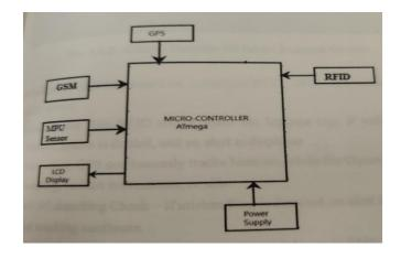
Figure 1: Data flow diagram of smart luggage system
