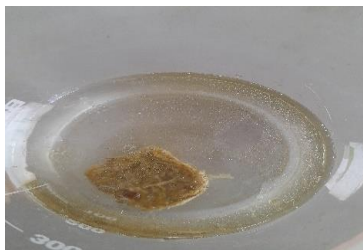
Fig6: Felt fibres after immersion in di-chloromethane
