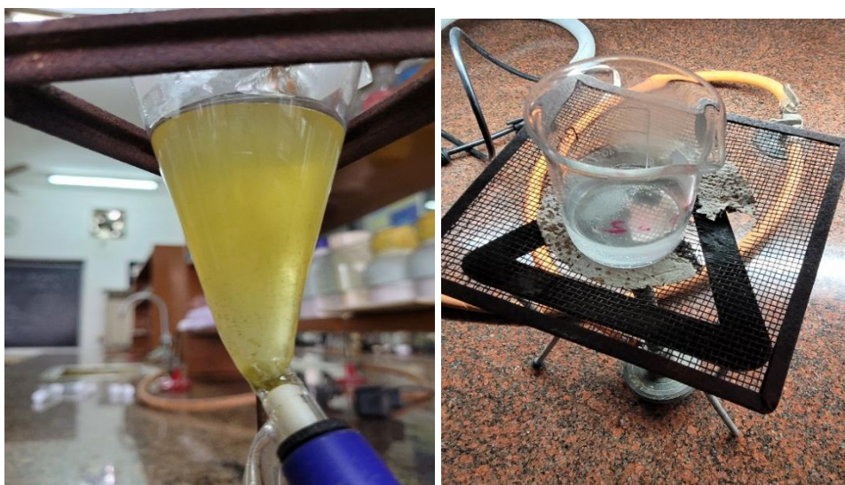
Figure 3: separation of volatile oil from aqueous phase
