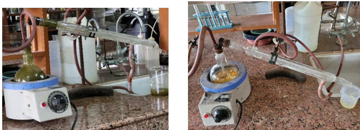
Figure 2: extraction of oil by hydro-distillation method
