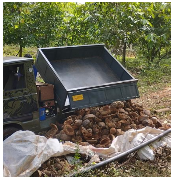
Figure 3: - Result of side dumping of dumper body.
