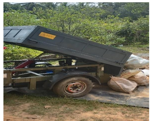
Figure 5: - Result of rear side dumping of dumper body.
