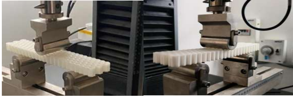
Figure 4: Experimental setup for mechanical testing of 3D-printed honeycomb structures under (a) compressive load and (b) three-point bending load using a Universal Testing Machine (UTM).
