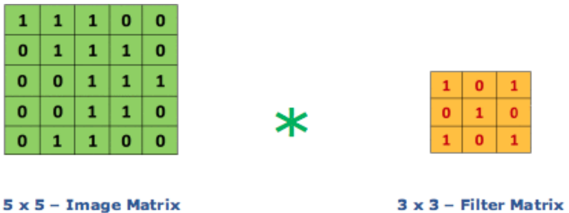
Fig 4.4.2: Image matrix multiplies kernel or filter matrix(2).
