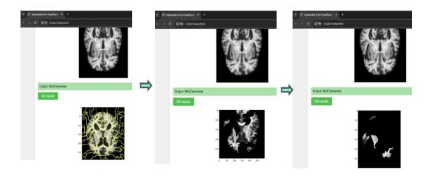
eXplainable AI (XAI) has been integrated using the SHAP (SHapley Additive exPlanations) to explain the predictions of a Convolutional Neural Network (CNN) model trained for image classification and Local Interpretable Model-agnostic Explanations (LIME) technique to explain the predictions of a pre-trained InceptionV3 model for image classification.
