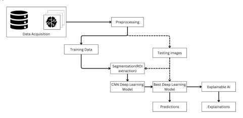
Project implementation starts with data acquisition, gathering relevant images for analysis, followed by preprocessing to refine and enhance the dataset's quality. Subsequently, the data is divided into training and testing sets, allowing a Convolutional Neural Network (CNN) to learn from the training data and segment regions of interest (ROIs) in the testing images.
