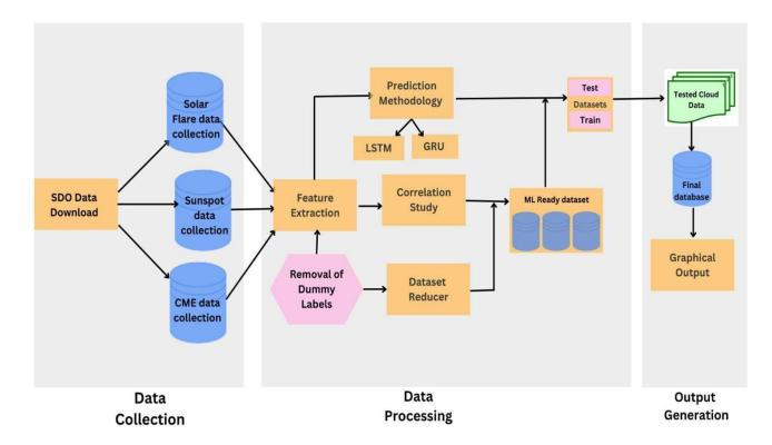
The methodology used involves a three-stage process related to solar flare prediction or space weather forecasting using machine learning techniques. This intricate process includes a series of steps aimed at collecting, processing, and generating insights from data to enhance our understanding of solar activities.
