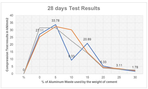
From the results and graphs of 28 days we can notice that the compression test results will increase till 5% replacement of cement by aluminum waste by the weight of cement.
