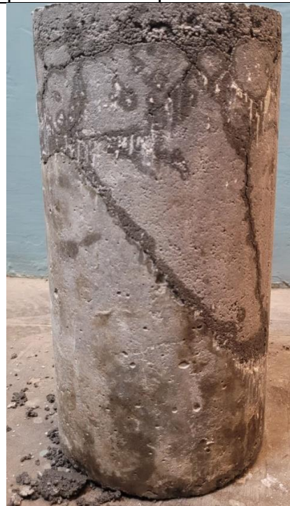
Fig: 22 Failure in the sika repair material bonded to substrate at predetermined plane of 45°
