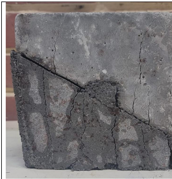
Fig:11 Interfacial failure between substrate and Asian paints repair material at predetermined plane of 30° along with vertical cracks
