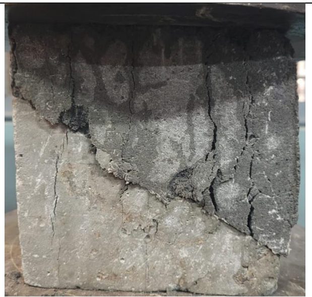
Fig: 12 Failure in the Asian paints repair material bonded to substrate at predetermined plane of 30°
