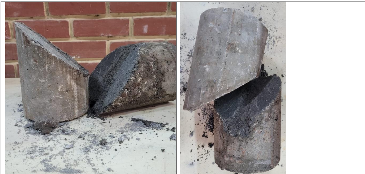
Fig: 19 Interfacial failures between substrate and Asian repair material at a predetermined plane of 30^\circ
