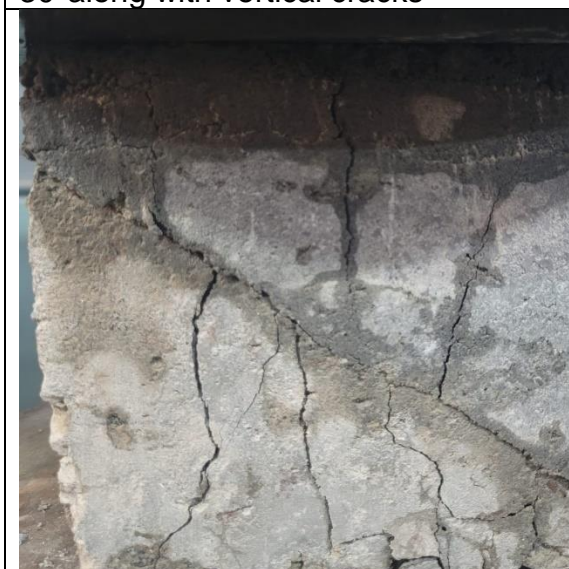
Fig:11 Interfacial failure between substrate and Asian paints repair material at predetermined plane of 30° along with vertical cracks
