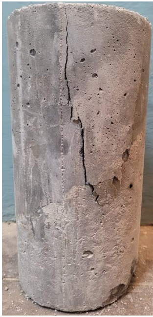
Fig: 21 Failure in the sika repair material bonded to substrate at predetermined plane of 30°
