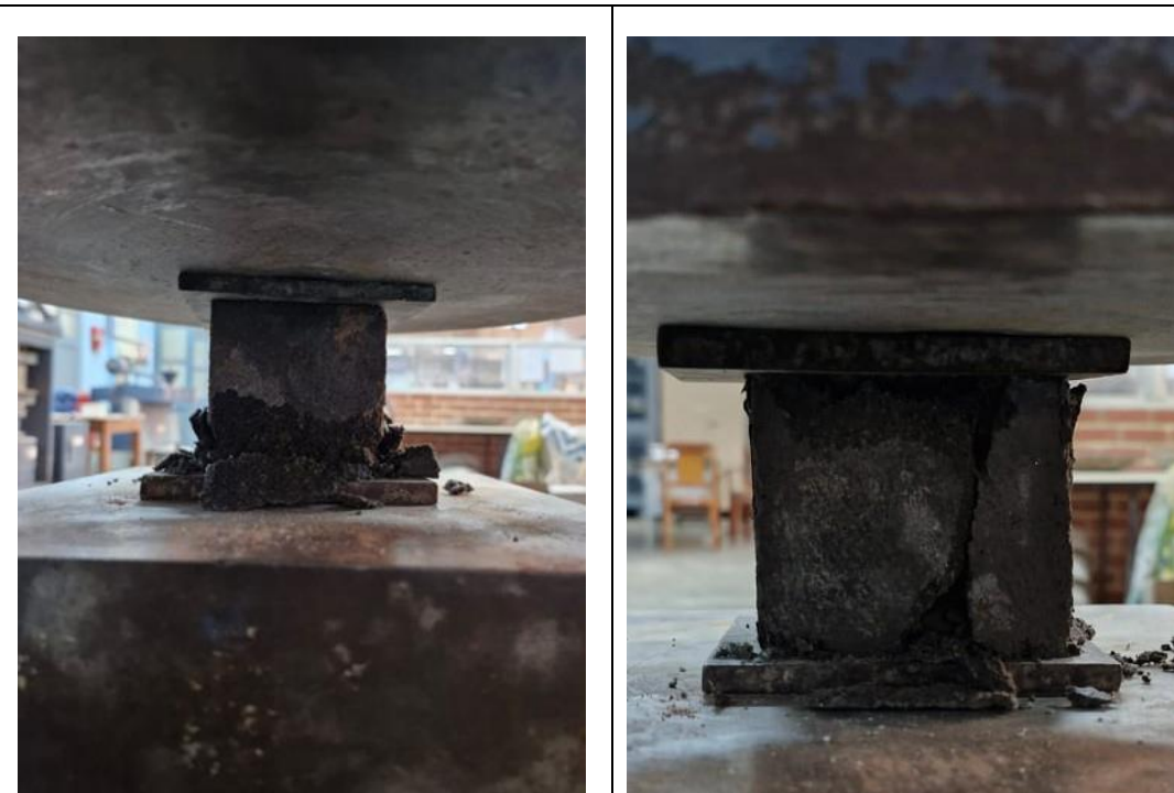
Fig: 6 Unsatisfactory failure of Blended mortar
