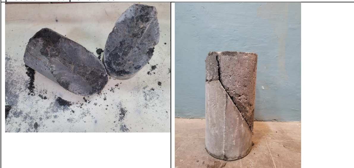
Fig: 20 Interfacial failures between substrate and Asian repair material at a predetermined plane of 45^\circ
