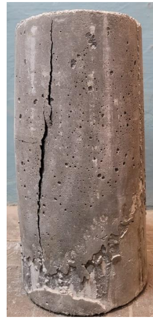
Fig: 22 Failure in the sika repair material bonded to substrate at predetermined plane of 45°
