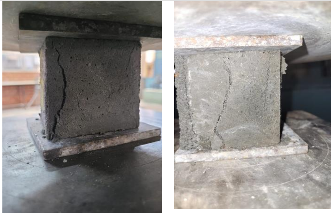
Fig: 5 Vertical failure of Sika latex power repair mortar
