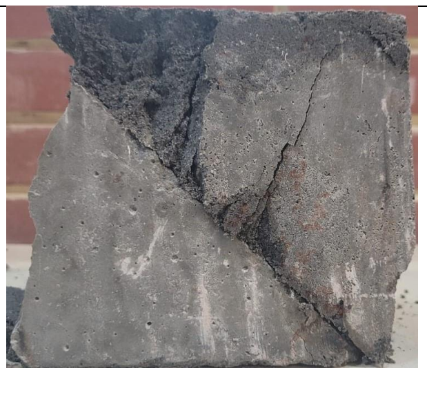
Fig: 12 Failure in the Asian paints repair material bonded to substrate at predetermined plane of 30°
