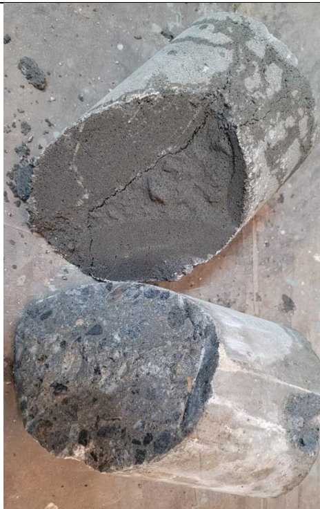
Fig: 23 Interfacial failures between substrate and PPC repair material at a predetermined plane 30°
