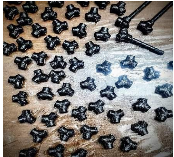
Fig.55: Resin infused roll wrapped 3D printed Y- connectors with carbon fiber threads
