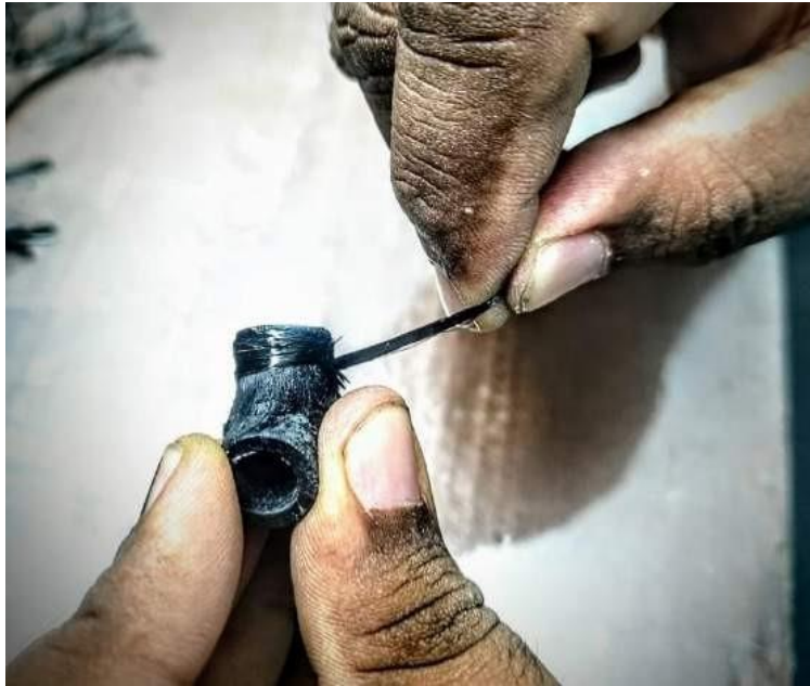
Fig.53: Roll wrapping of 3D printed Y- connectors with carbon fiber threads
