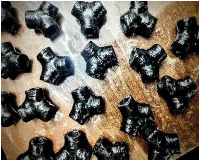
Fig.55: Resin infused roll wrapped 3D printed Y- connectors with carbon fiber threads
