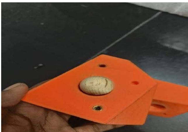
Fig.48: Placing / positioning the wooden ball in 3D Printed Jigs for drilling
