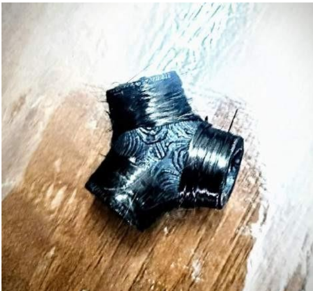
Fig.54: Roll wrapped 3D printed Y- connectors with carbon fiber threads
