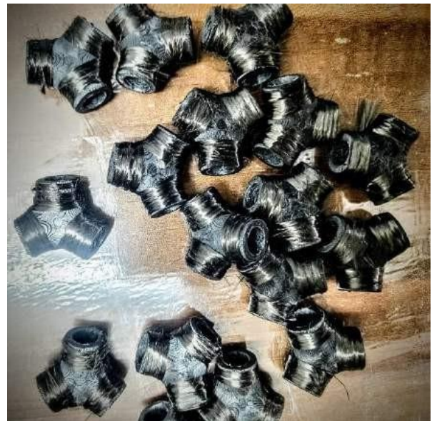
Fig.54: Roll wrapped 3D printed Y- connectors with carbon fiber threads
