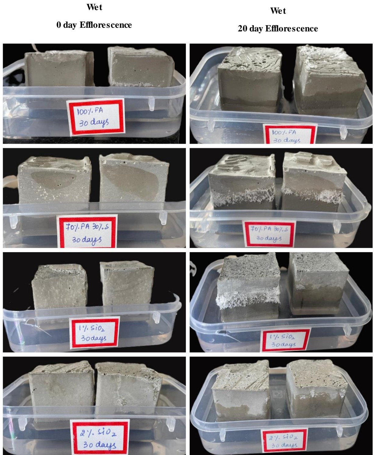
Figure 2. Efflorescence of 0 day and 20 day aged geopolymer specimens when stored with the bottom in contact with water
