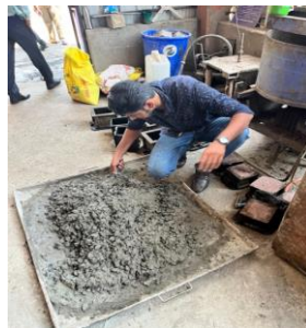
Cubes casted for Carbon fibre reinforced concrete
