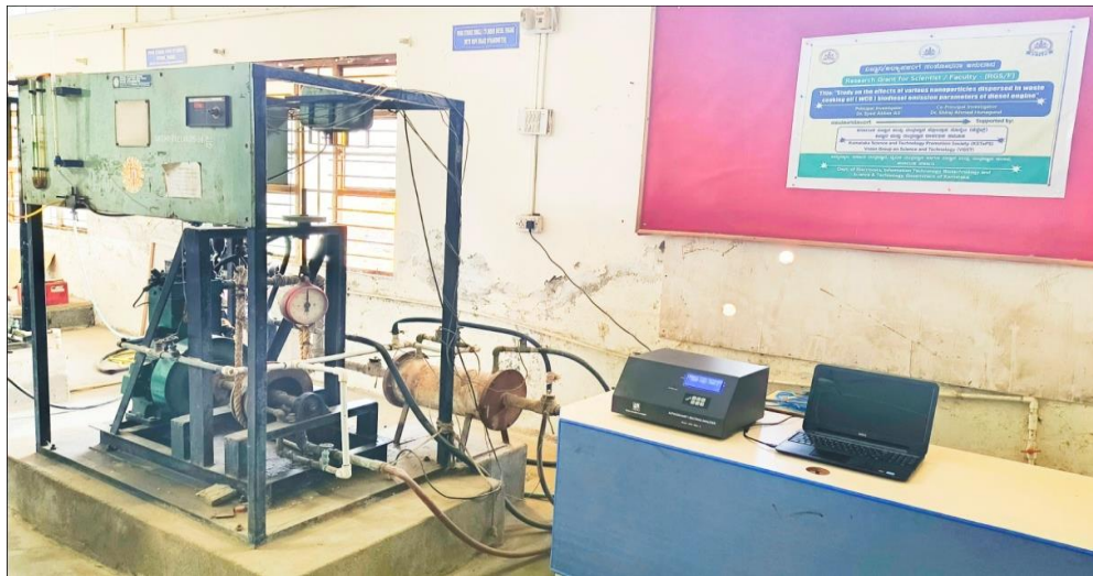
Fig. 4: Four Stroke Diesel Engine Test rig and Emission Analyzer
