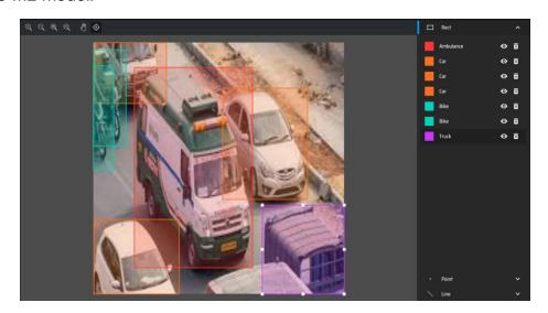
**3. YOLOv8 Model:** YOLO stands for You Only Look Once. It is used for Object Detection which involves identifying and localising objects within an image or a video frame.
