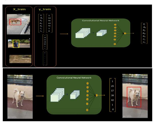
**4. Training the ML Model:** Train the YOLOv8 model on the annotated dataset using Google Colab. Around 14000 images are used for training and 3000 images for validation. Additionally, the hyperparameters which include learning rate, batch size, and number of epochs are tuned to optimise model accuracy and reduce losses.
