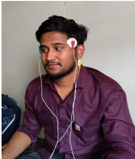
Figure 5.1: Collection of Mind Data using EEG Sensor, Figure 5.2: Displaying the EEG data.
