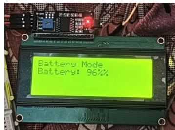
Fig:1 System in battery mode monitoring the battery level
