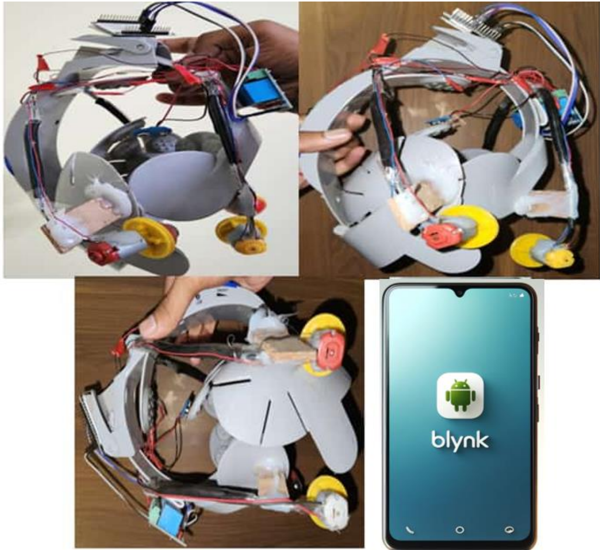
Fig. 6.1: Shows a working prototype model of a head massaging device.
