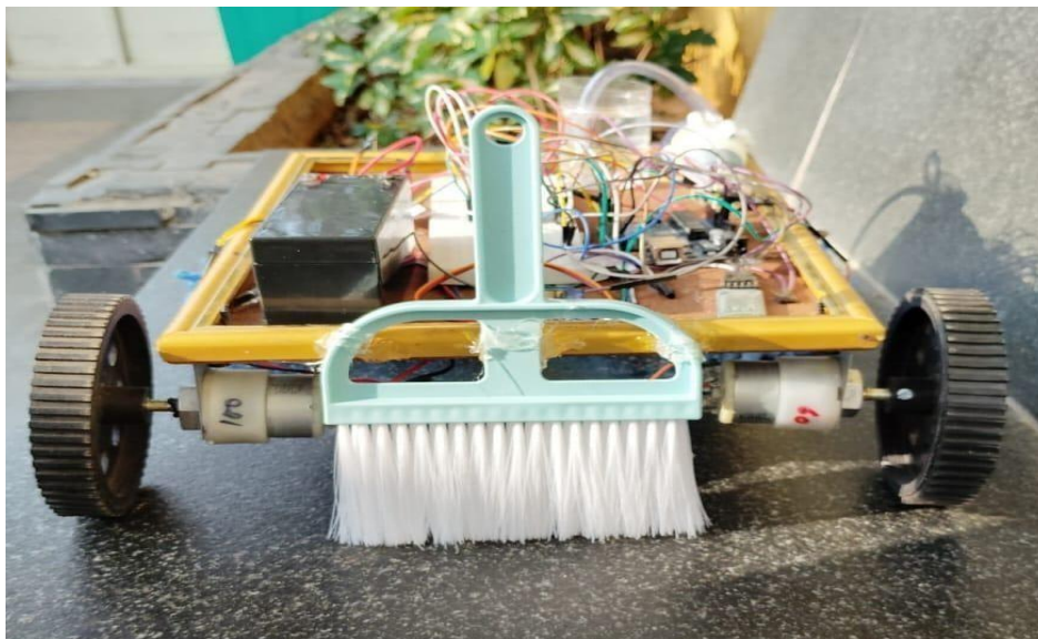
Figure 4: Cleaning Robot Sweeping Section
