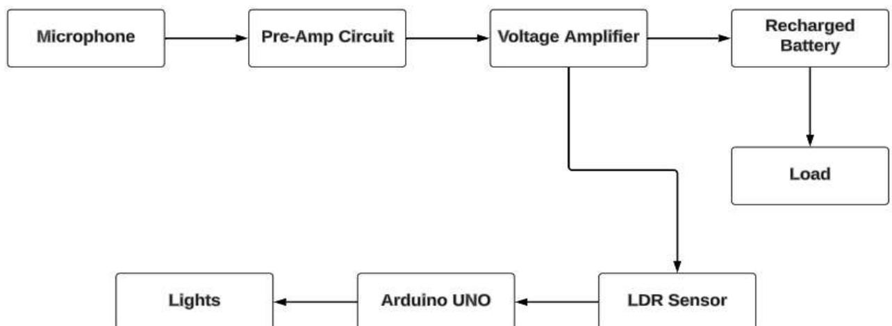
Working flow of Block Diagram:
