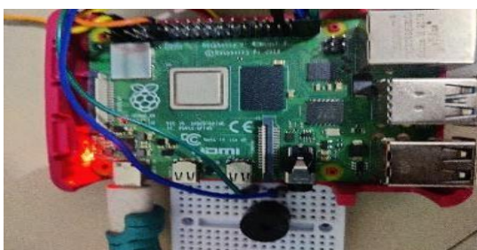
Figure 3: Circuit connection of Raspberry Pi with piezo Buzzer and Servomotor
