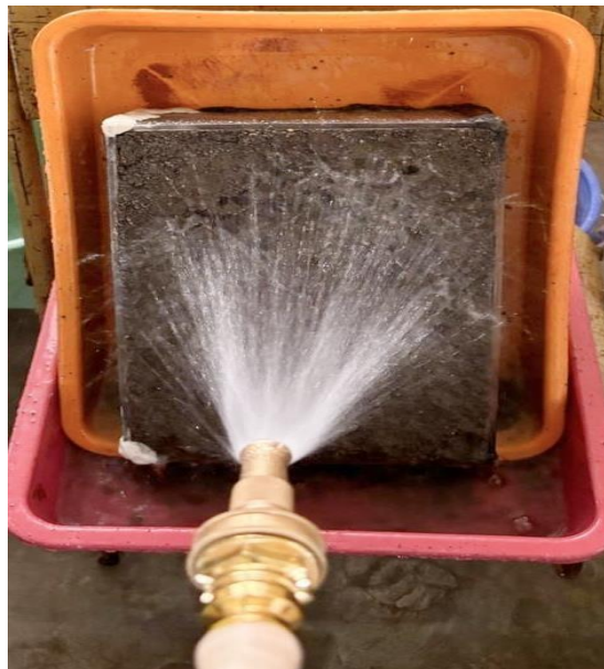
Fig 4.6 Rainfall simulation (slope subjected to rainfall intensity of 45 mm/hr)
