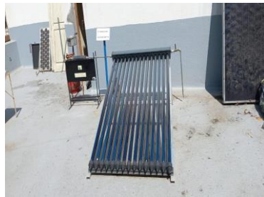
Fig 4 Hybrid Solar cooking system
