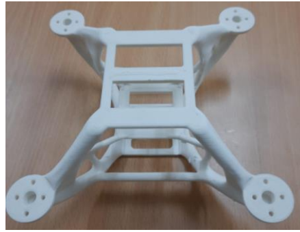
Figure 4:-D printed frame using PLA
