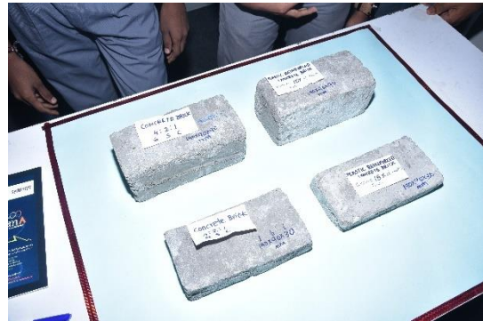
Fig 14: Bricks with different Plastic composition
