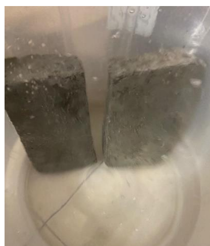
Fig 18: Bricks immersed in water for 24 hours
