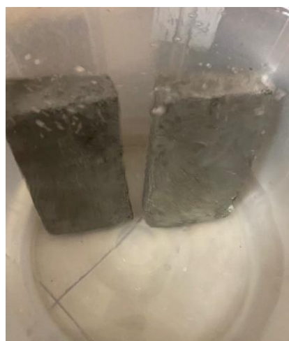
Fig 17: Water Absorption Test
