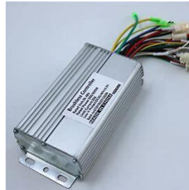
Fig.6 BLDC Electric Motor Controller
