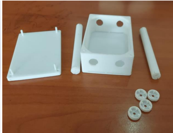
Proposed model and 3d printed case for the damper system
