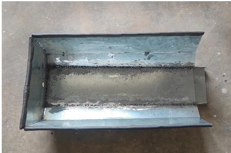
Fig. Fabrication of collection tank
