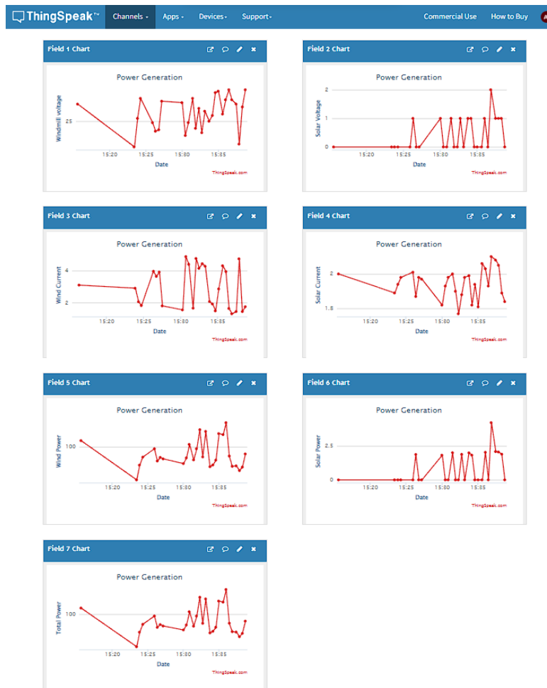
Figure 2: Voltage, current and power readings uploaded to ThingSpeak
