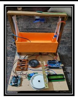
The above figure represents the proposed model of the system where it aims at monitoring the baby. When the Sound sensor detects the cry of the baby in the cradle, the sensor will sent the signal to the arduino uno, and depending on the input, the output is activated and voice recorder is active along with the relay, the relay is used to on the gear motor, which is used to swing the cradle.
