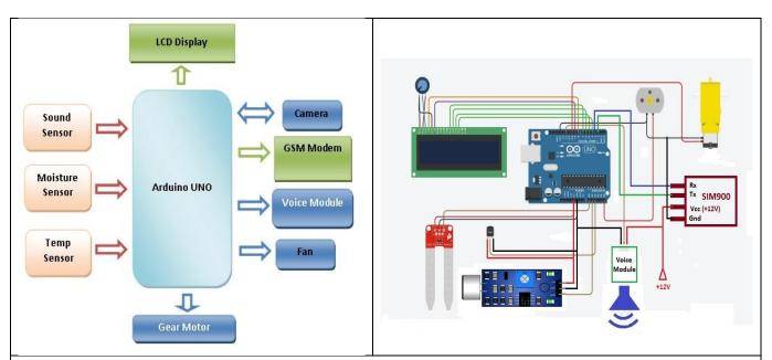
The sensors are the main source of input to the Arduino. Based on the three sensors' input, microcontroller sends three different messages respectively, the messages that have been received to the mother's official's registered mobile number.
