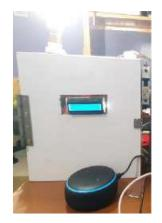
Above Figure shows the Smart Energy Meter Pv2 in action with Alexa Speaker. The bulb on the device is the dummy load used to test the device. The bulb is turned on by giving a voice command to Alexa.
