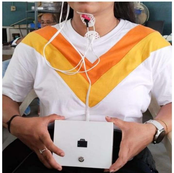
Fig 6.2.1 BREATH AND SWALLOW SENSING ON OLED WITH ELECTRODES FOR EMG SENSING
