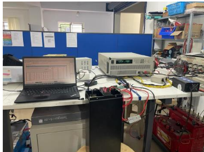
Fig: Charge -Discharge Test experimental setup
