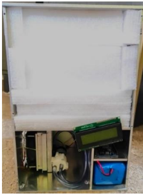
Figure 4. Internal compartments of the refrigerator
