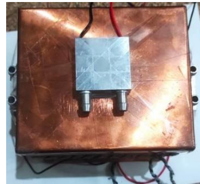
Figure 5. Copper container with Peltier sensor
